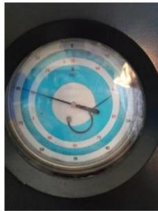
Gambar 1. Indikator Hardness
