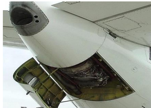
Gambar 1. Auxiliary Power Unit
