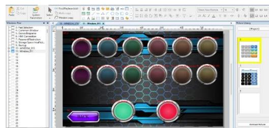
Gambar 7. Tampilan HMI Lampu Flip-Flop
