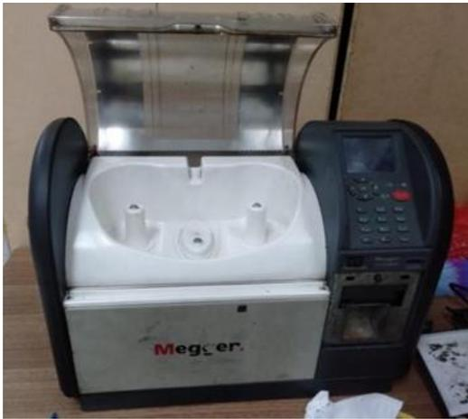
Gambar 3. Alat Uji Breakdown Voltage (BDV)
